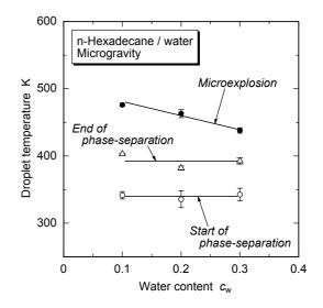
Fig.1 Droplet temperature at start and end of phase-separation and at microexplosion.
