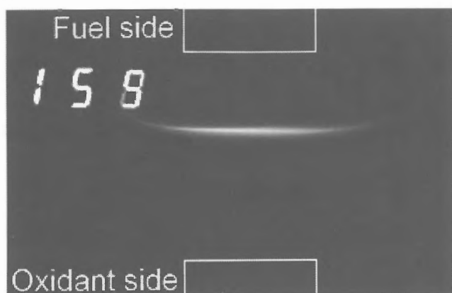
Fig.1 Direct photograph of counterflow diffusion flame. ( \epsilon = 4.53 \text{ s}^{-1} , Fuel: C 3 H 8 , T = 700 K)
